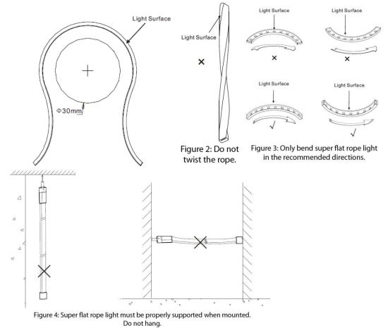
2. Super Flat Rope Light can be cut every six or ten LEDs, depending on the color, at specific cut points. Dotted lines on the back side of the rope indicate where cuts can be made. Be sure your cut is a straight line, perpendicular to the rope light, as shown below.
