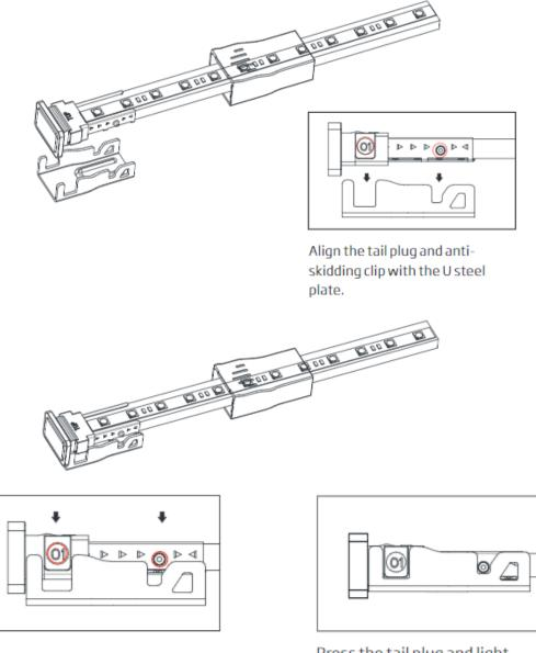
Press the tail plug and light downwards at the same time till bottom.
