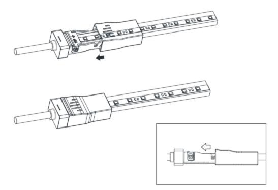
Slide back the PC cover till it snaps in the feed connector.
