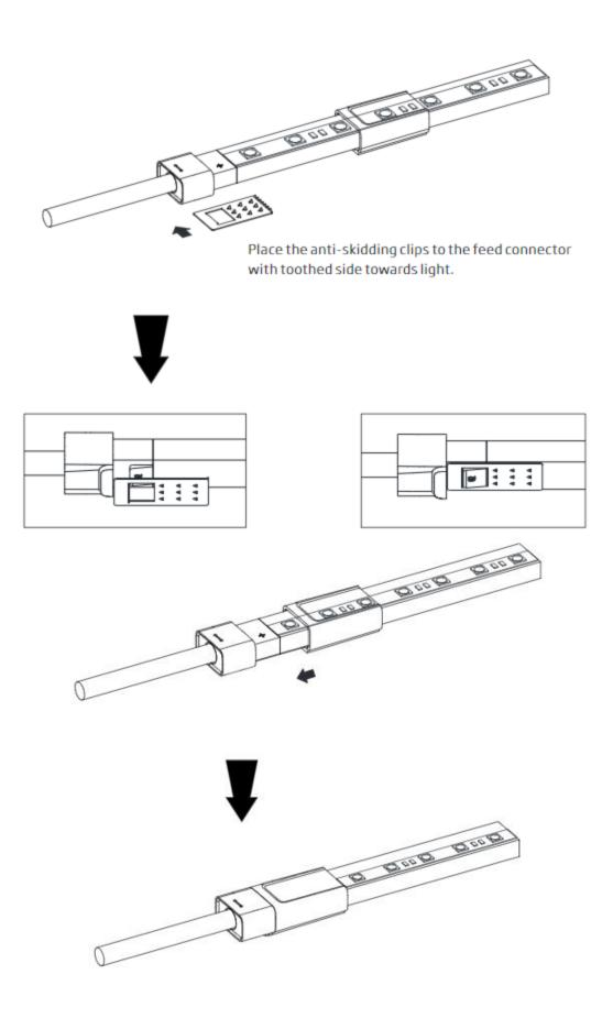
8. Proper assembly of 40 series end cap.
