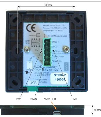
**PORT** : Scratch away sticker over 2 dots shown. Solder wires to the exposed solder points. Connect these to trigger a single scene to start
