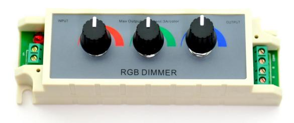
The three channel LED dimmer is an easy way to mix colors with any 12 or 24 volt RGB LED product. Apply the correct DC voltage to the inputs and the controller will generate pulse dimming signals on three separate output channels (red, green and blue).
