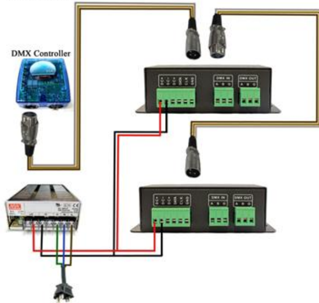
DMX512-PX Decoder Daisy Chain Wiring Diagram
