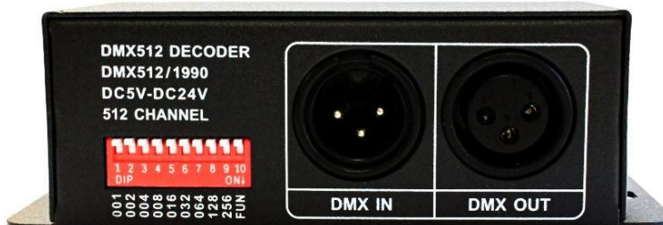
Figure 1: DMX512 Input (3-pin) and DMX serial OUT port
