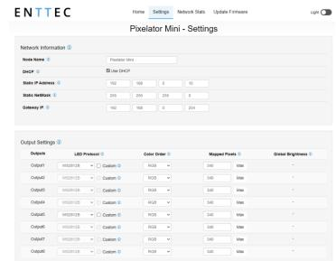
The PIXELATOR MINI provides more than 20 output SPI (Pixel) protocols listed below:
