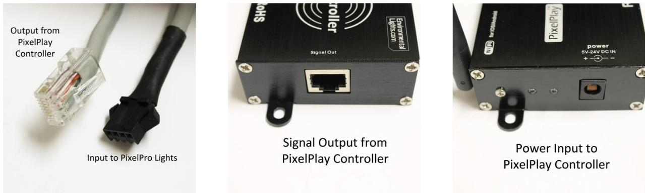
Use the included connector cable to plug your PixelPro lights into the “Signal Out” port of the PixelPlay controller. Up to 500 pixels can be connected, although it is necessary to inject power as listed below in order to avoid voltage drop and discoloration or dimming of your lights.
