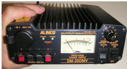
A back-lit front panel meter indicates voltage and current. Light-duty accessories can be powered by two pairs of 5 amp spring terminals, a 10 amp cigarette lighter jack, or the husky 32 amp rear-panel terminals. The front-panel voltage control has a midpoint detent set to deliver nominal 13.8 VDC to emulate the mobile DC environment for typical base/mobile radios.
