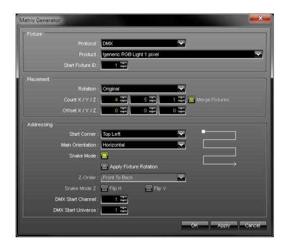
• In theory, the LEDs are arranged as follows: 3 pixels per LED [due to RGB], 4 fixtures per row, and a total of 5 rows. Please see the picture below:
