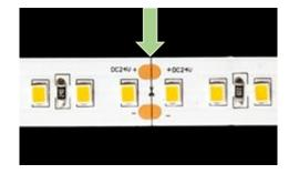
Waterproof LED strip light can be cut in the same way as non-waterproof LED strip. The difference is that it needs to be resealed at the cut end to maintain the waterproof rating. The waterproofing process is fairly simple, but it is very important to follow all of the steps to ensure a good seal. Improper waterproofing can cause LED strip failures in the field. Please view our video on waterproofing strip light for more details.
