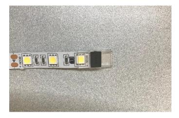
3. Repeat for the opposite side. If using LPL-X, just slide the wires into the connector, making sure to line up the wire with the piercing points.
