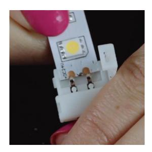
3. Close the gate. When the gate locks. It should lock make an audible sound.
