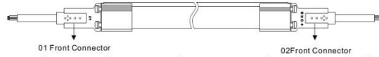
Figure 8: If powering from one end, maximum run length is 10m (33 feet). If powering from both ends, maximum run length is 20m (65 feet).
