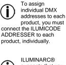
ILUMINARC® suggests that you connect no more than 20 products in this mode and keep the total distance to less than 60 m (197 ft). Otherwise, you might need to use an optically isolated signal amplifier.
