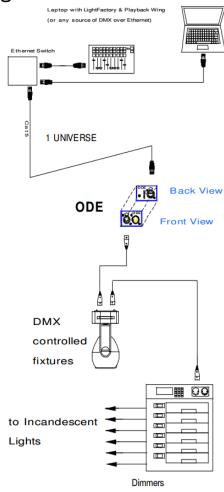
**\*Note:** if you plan to connect two ODE's together without entering a network switch, a crossover cable will be required.
