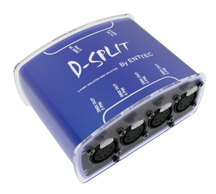
D-SPLIT is an optical isolator/splitter for DMX512. Its purpose is to allow the user more flexibility in connecting their DMX controlled devices.
