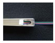
6. Put electrical tape on the back of your lights to electrically insulate the strip from the metal channel. If you chose the RGB rigid strip, put 3 thicknesses of electrical tape over the solder bumps protruding through the back of the strip or the pointy bumps will poke through the tape and the channel will short your lines together.
