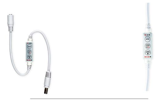
The MiniLine Dimmer is an easy-to-use and versatile inline dimmer for use with any of our one-channel LED products. Simply connect your power supply and single-channel LEDs to the MiniLine Dimmer. Power-off memory returns the MiniLine to the settings last used if power is removed. Use the built-in lock-out mode to secure your settings.
