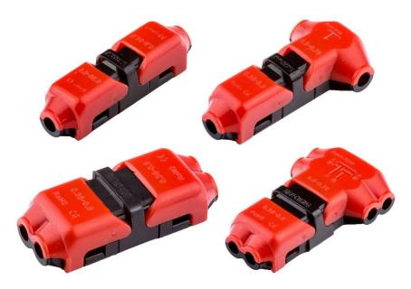
Clip-On connectors from Environmental Lights are a quick and easy way to connect segments of wire, no soldering or wire stripping required. The connectors use angled metal contacts that slice through the wire jacket without cutting the actual wire. All models accept 18-22 AWG stranded wire (0.6-2.1mm). They are rated for 9-Amps of continuous current for each contact and have an absolute maximum of 10-Amps. Clip-On connectors are intended to make permanent connections.
