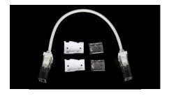
This is a 2-wire, IP67 jumper designed to connect two sections of Eluxtra™ ProFlex LED strip lights that have been cut to custom lengths. Look for the "01" and "02" markings on your strip light to ensure you are connecting in the proper direction.
