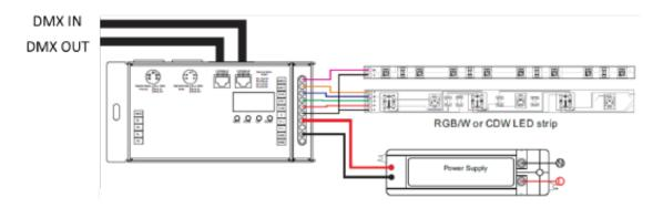
b. **12 Channel Decoder**: Connect the LEDs and power supply using the screw terminals. Power supply positive and ground should be connected to "V+" and "V-" terminals respectively. LED positive should be connected to the "+" terminals. Connect LED negatives to output channels 1-12 as appropriate for the installation.
