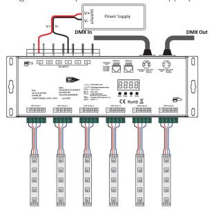
d. **25 Channel Decoder**: Connect the LEDs and power supply using the screw terminals. Power supply positive and ground should be connected to "V+" and "V-" terminals respectively. LED positive should be connected to the "+" terminals. Connect LED negatives to output channels 1-25 as appropriate for the installation.
