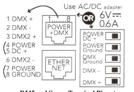
**RJ45 and Screw Terminal Pinout**
