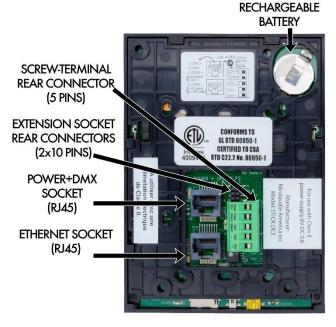
• Screw Terminal Connector – Used to connect DC power and output DMX universe 1. The pinout is shown below.
