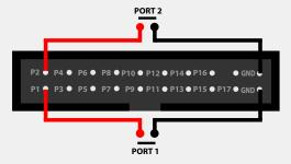
To activate a port, a brief contact of at least 1/25 second must be established between the ports (1...16) and the ground (GND) using the external HE20 connector. Note: the scene will not be switched off when the switch is released.
