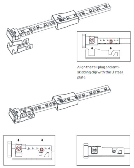
Press the tail plug and light downwards at the same time till bottom.
