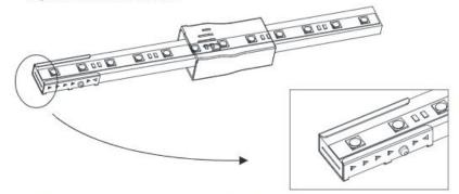
Fit the anti-skidding clip to the end of the light so that it wraps tightly and its brim is aligned with the cut edge on both sides.
