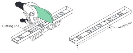
Cut the light only at printed cutting line with printing mark face upwards
