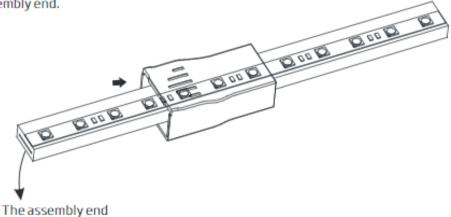
2. Install the anti-skidding clip onto the neon ensuring that it lines up with the cutting edge.
