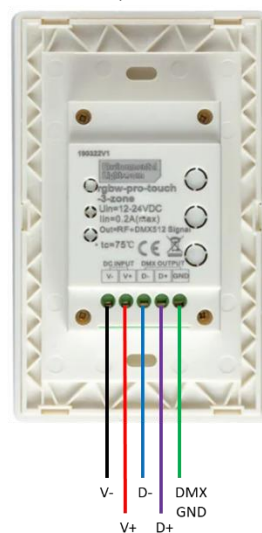
Wiring for DMX Use (with or without Wireless)
