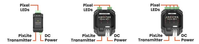
When connecting to a **PixLite T8-S Mk3**, pixels are connected as follows:
