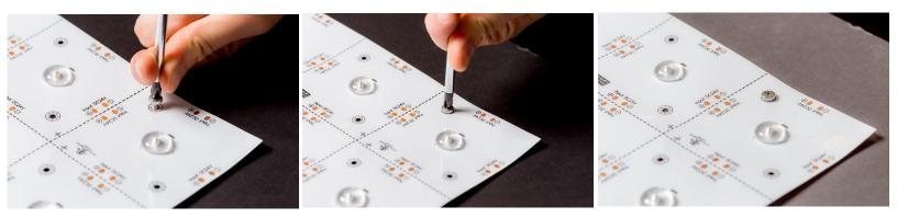
b. <u>Adhesive</u>: To use the adhesive backing, peel back the paper layer on the back of the sheet. Properly clean any surface of dust before applying the sheet. Press the light sheet down and hole firm for 10 seconds to ensure a long-lasting attachment.
