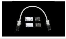
This is a 4-wire, IP68 jumper designed to connect two sections of Eluxtra™ ProFlex LED strip lights that have been cut to custom lengths. Look for the "01" and "02" markings on your strip light to ensure you are connecting in the proper direction.
