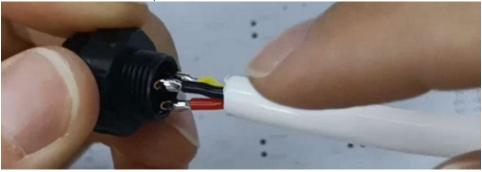
NOTE: Ensure that the wires on the male and female sides match.
