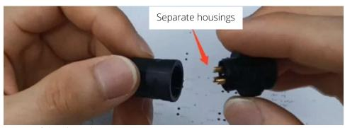
1. Loosen the locking nut of the plastic housing.
