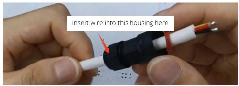
a. NOTE: make sure the waterproofing silicone ring remains in the plastic housing. If it falls out, place the ring over the wire as shown below.
