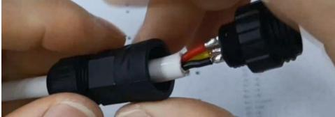
6. Tighten the housing to the pin connector then tighten the locking nut.
