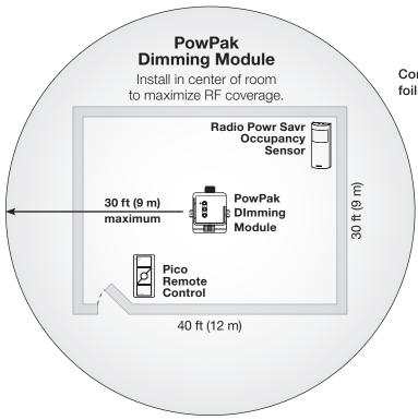
Contact Lutron first for applications using foil-backed or metallic ceiling tiles.
