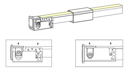
Press the tail plug and light downwards at the same time till bottom.
