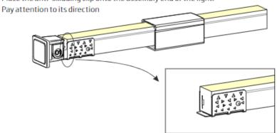
Fit the anti-skidding clip to the end of so that it wraps tightly and its brim is aligned with the cut edge on both sides.
