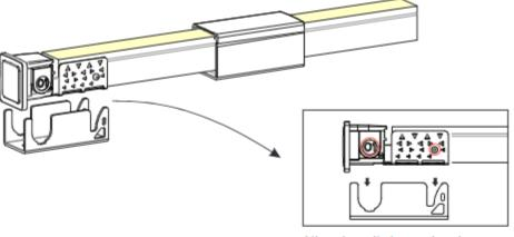
Align the tail plug and antiskidding clip with the U steel plate.
