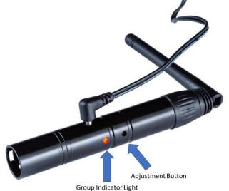
3. Press the recessed Adjustment Button to change the grouping of the transmitter. The group will be indicated by the Group Indicator Light. All receivers with the same color Group Inidicator Light will be controlled by the transmitter. The EasyWireless transmitter and receiver come with seven groups allowing for up to 7 separate transmitters in the same installation.
