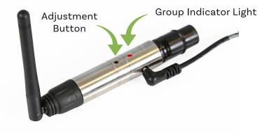
3. Press the recessed Adjustment Button to change the grouping of the transmitter. The group will be indicated by the Group Indicator Light. All receivers with the same color Group Inidicator Light will be controlled by the transmitter. The EasyWireless transmitter and receiver come with seven groups allowing for up to 7 separate transmitters in the same installation.
