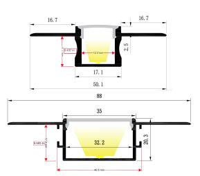
Stick LEDs in the aluminum housing.
