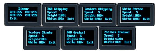
Selecting the "Test" menu enters stand-alone mode. The decoder will ignore any DMX inputs when in this mode. The dimmer function will set a static color by setting the DMX values for each channel independently. Values range from 0-255. All other modes have adjustments for speed, RGB brightness and white brightness. Exit will return to the main menu and end standalone mode.
