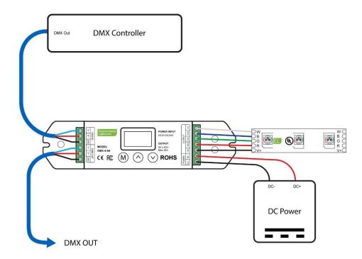
4. For DMX control: Connect the outputs of the DMX controller to the "D+", "D-" and "GND" terminals for "DMX IN". Additional DMX devices may be connected using the "DMX OUT" terminals. Only apply a DMX signal while the decoder is powered on.
