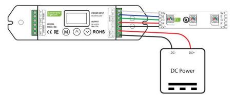
3. The DMX terminals do not need to be connected for operation in stand-alone mode
