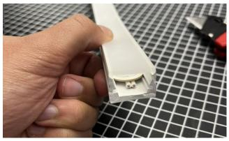
5. Ensure the end cap is dry, apply ample glue to the inner surface of cap, and line up end cap with sheath. (We recommend our waterproof glue: sf-glue)
