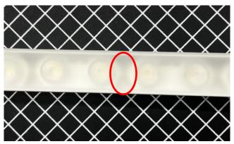
3. Cut through the outer sheath first and separate the sheath to expose the inner modules and wires between modules.
