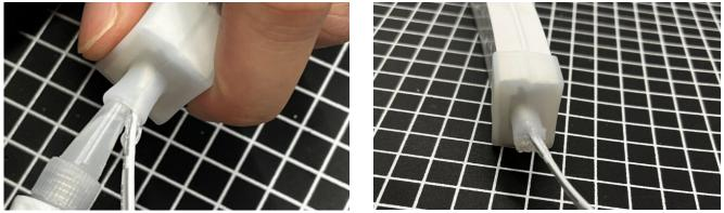
11. Allow the glue to dry (at least 24 hours) before installing and powering the strip.
