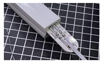
\*Note: If you are using a lead with a connector that won't fit through the end cap hole, please feed the end cap onto the wire before soldering\*\*
