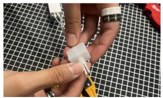
9. Apply more glue to the inner part of the cap, ensuring the glue coats the wires and line up the end cap with the sheath.
