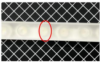
3. Using a sharp knife or shears, cut through only the outer sheath first and separate the sheath to expose the inner modules and wires between modules.
