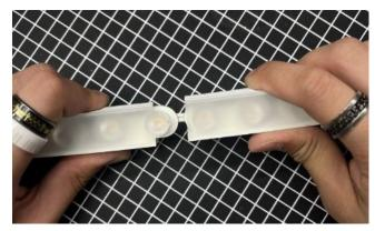
4. Cleanly cut wires between modules. Ensuring that there are no stray wire strands that could cause a short between two conductors.
