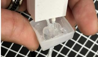
10. Secure the end cap to the sheath and apply glue to the cap, filling the wire exit to ensure a waterproof seal.
