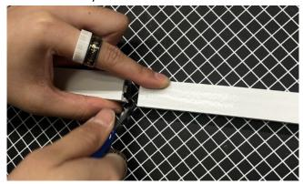
5. Using needle nose pliers or a similar implement, carefully pull the module out enough to access the wires. Hold the module in place while performing the next steps; otherwise, the module will recede back into the sheath.
