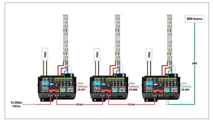
**Note:** The CVC4 allows for operation mode to be set by DIP Switches only – Not via RDM.
