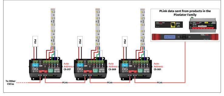
**Note:** when using CVC4s with any product within the Pixelator Family, set the P-Link port you have connected your CVC4s to output WS2812b with colour ordering **RGB**. This will convert your input DMX signal 1:1 into P-Link allowing you to mix and match CVC4 operating modes within the same String and patch them within your lighting control software.
