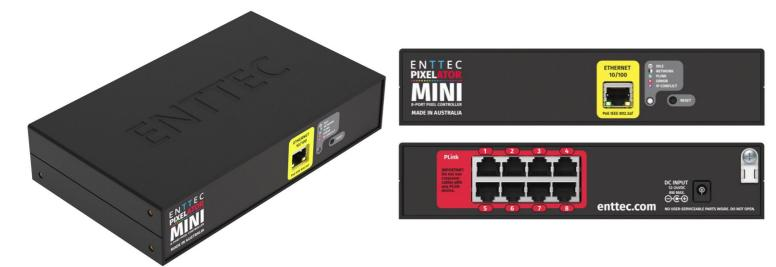
ENTTEC's PIXELATOR MINI is an 8-port Ethernet pixel controller. Using ENTTEC's PLINK protocol, each port provides data to ENTTEC's PLINK INJECTOR which can control up to 2 Universes each, making the PIXELATOR MINI powerful enough to control up to 8,192 channels (2,730 RGB Pixels) with perfect synchronization across all eight of its outputs.
