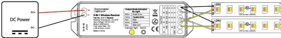
For single color, connect each wire to a separate channel on the receiver. The positive wire connects to the V+ terminal. Once connected, press the switch button until the indicator light shows white.
