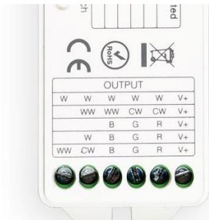
For 5 channel control, connect red to R, green to G, blue to B, cool white to CW and warm white or amber to WW. The positive wire connects to the V+ terminal. Once connected, press the switch button until the indicator light shows blue.
