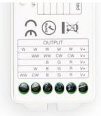
For 5 channel control, connect red to R, green to G, blue to B, cool white to CW and warm white or amber to WW. The positive wire connects to the V+ terminal. Once connected, press the switch button until the indicator light shows blue.
