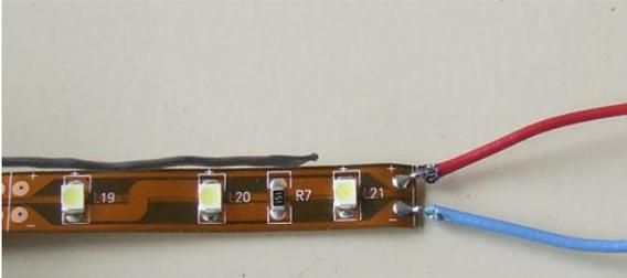
4. Carefully clip excess wire away from the back of the ribbon to ensure no short circuits.
