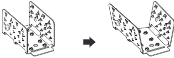
Unfold the anti-skidding clip about 20 degrees on both sides.
