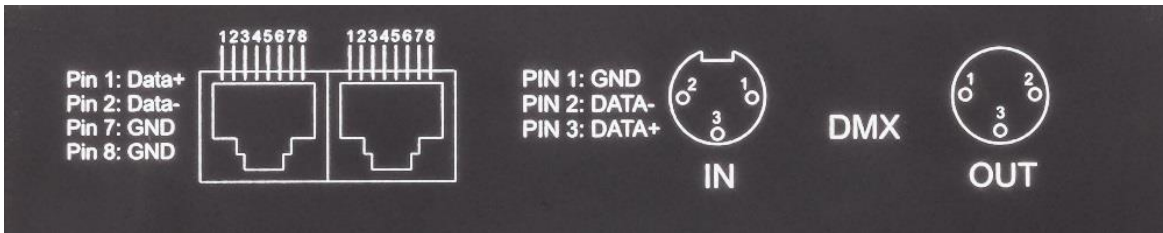
Figure III: Connector Pinout for DMX-4-5000-3-10A
