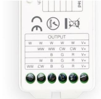
For 5 channel control, connect red to R, green to G, blue to B, cool white to CW and warm white or amber to WW. The positive wire connects to the V+ terminal. Once connected, press the switch button until the indicator light shows blue.
